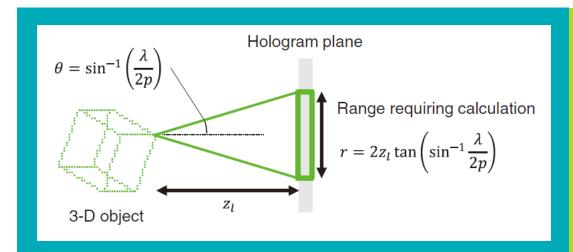
Range-dependent calculation: Limited by the pixel pitch of p the SLM
