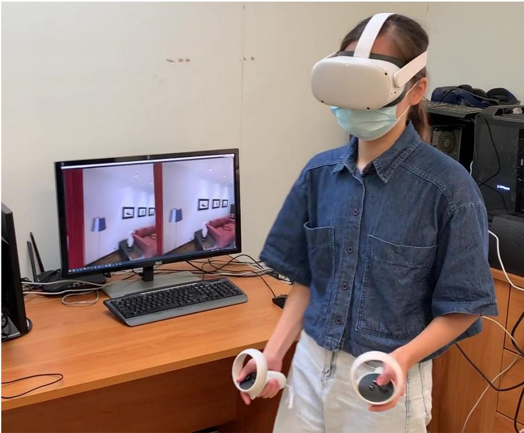
Figure 1.1: A VR user interacts with a VR application via the HMD and two hand-held controllers.
