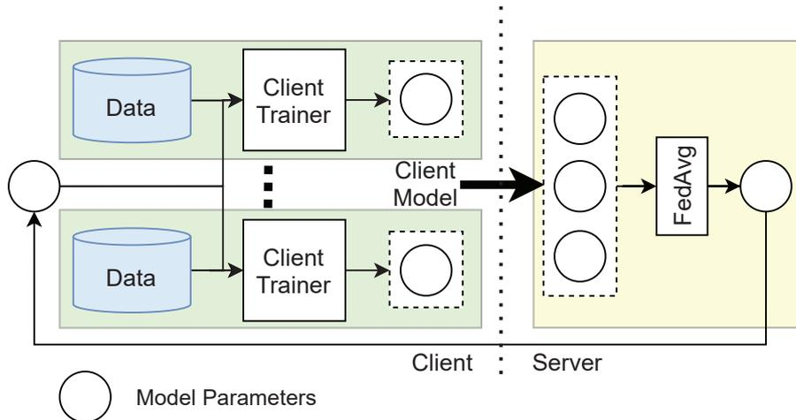
Figure 2.2: Federated learning using the FedAvg algorithm.
