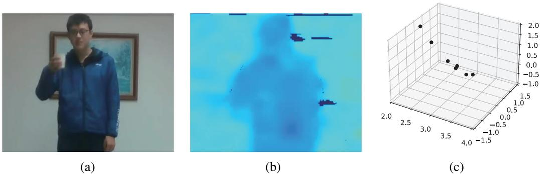
Figure 1.1: Sample data from: (a) an RGB camera, (b) a depth camera, and (c) a mmWave radar.
