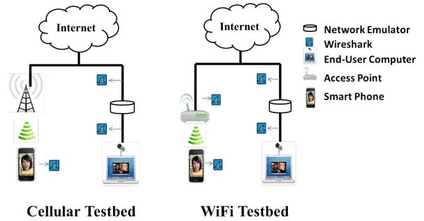
Fig. 1. Testbeds for Mobile Video Call Measurement
