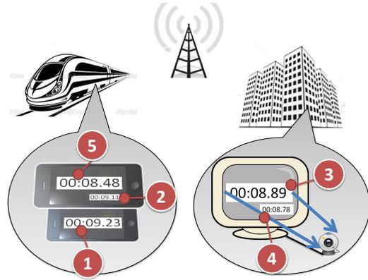
Fig. 3. Round-trip video delay testbed on subway.
