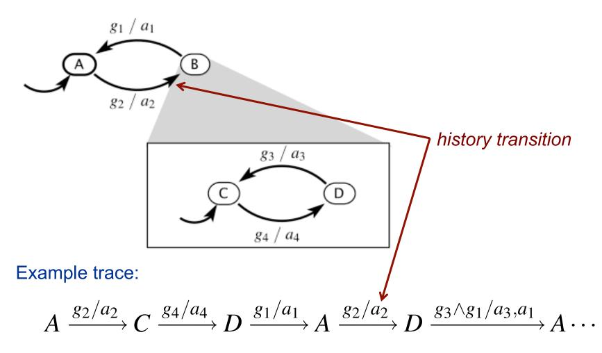
A history transition implies that when a state with a refinement is left, it is nonetheless necessary to remember the state of the refinement.
