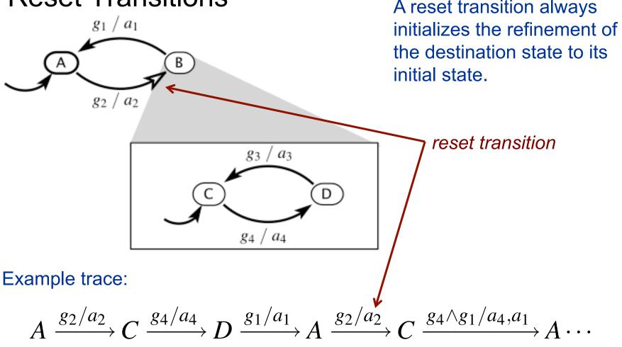
A reset transition implies that when a state with a refinement is left, you can forget the state of the refinement.
