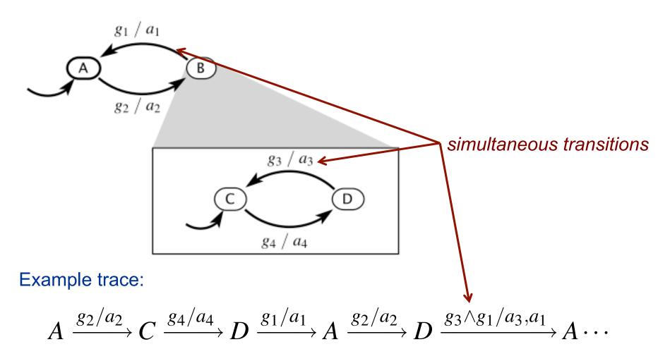
Simultaneous transitions can produce multiple outputs. These are required to not conflict.
